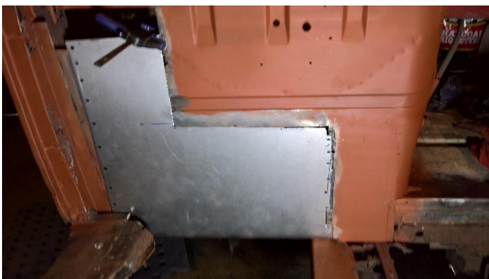
Seat tub with new piece
