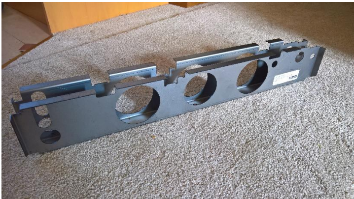
What a new front cross member looks like (hopefully to be fitted soon)
